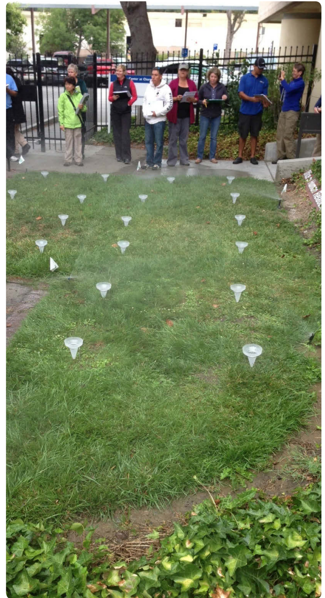
Catch can test during workshop.
