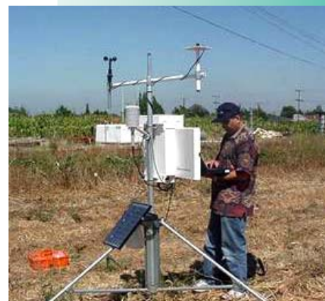
The District owns and maintains two CIMIS weather stations which provide growers with information to make efficient water scheduling decisions.
