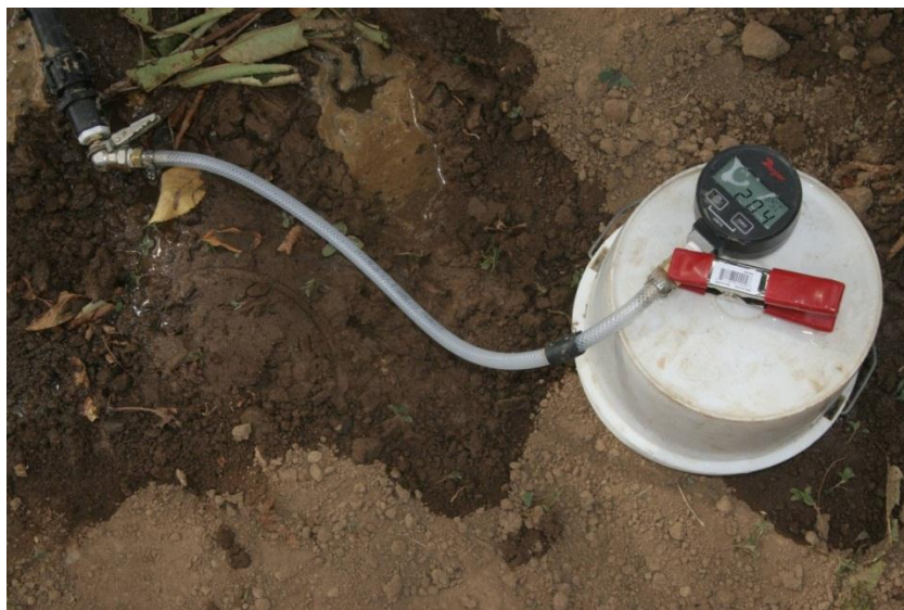
Evaluating the pressure at the end of a dripline
