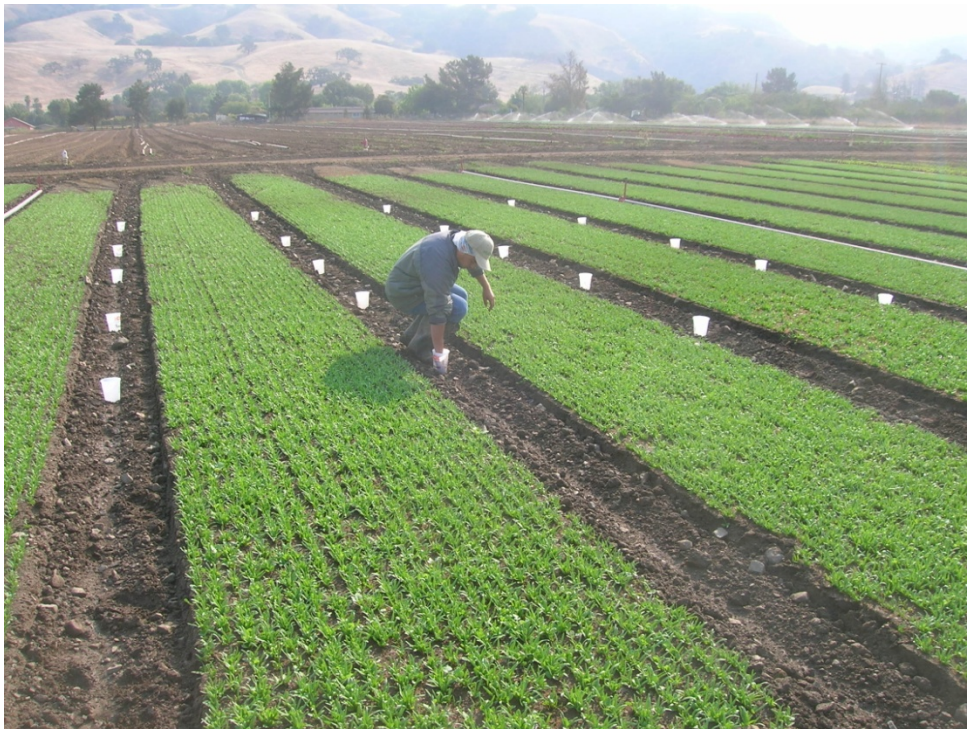
Figure 3. Irrigation evaluation of a solid set sprinkler system on baby leafy greens
