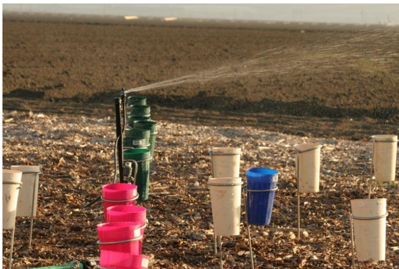
Sprinkler Testing at UCCE office
