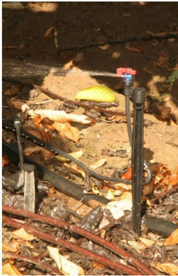
Nelson (left) & Netafim (right) rotating microsprinkling models tested
